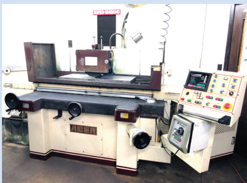
Acer Model Supra 1640AHD Surface Grinder
