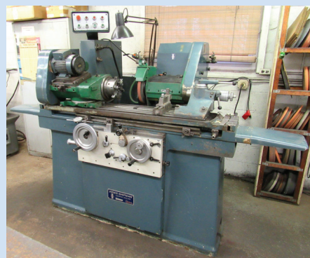
Jones & Shipman Model 1300EIU Cylindrical Grinders
