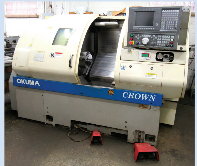
Okuma Crown L1060 Model 762S-BB Turning Center
