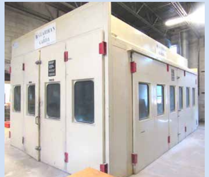
Guardian Garda Enclosed Paint Booth
