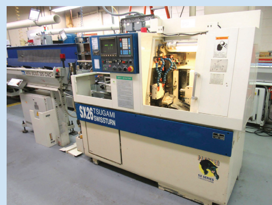
Tsugami Type BS26 CNC Multi-Axis Automatic with IEMCA Type Mini Boss 325 CNC Bar Feed
