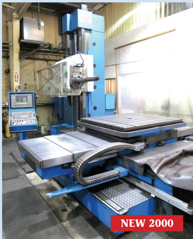
TOS Type WH105CNC 4.12" Table Type 4-Axis CNC Boring Mill
