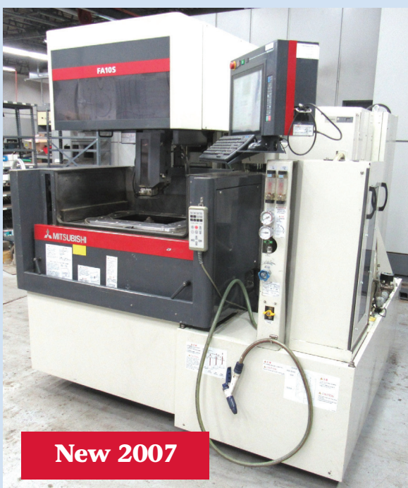
Mitsubishi Model FA10S Advance CNC Wire EDM Machine w/System 3R B-Axis Macro Rotary Table
