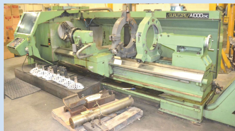
Gurutzpe Model A1000 40" x 120" Flat-Bed 2-Axis CNC Lathe
