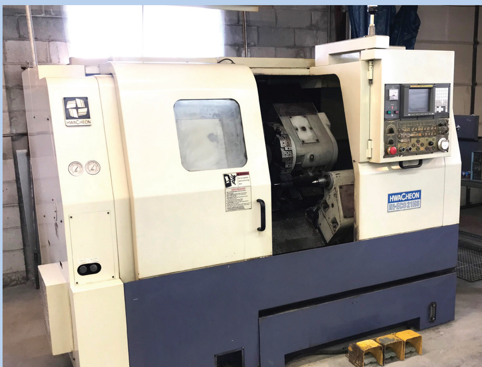
Hwacheon Hi-Eco 21HS CNC Turning Center with Fanuc 18i-T Control
