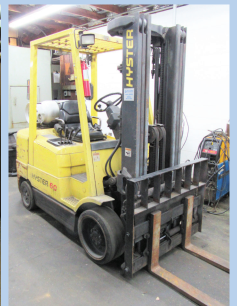
HYSTER Model S60XM 6000# Propane Forklift
