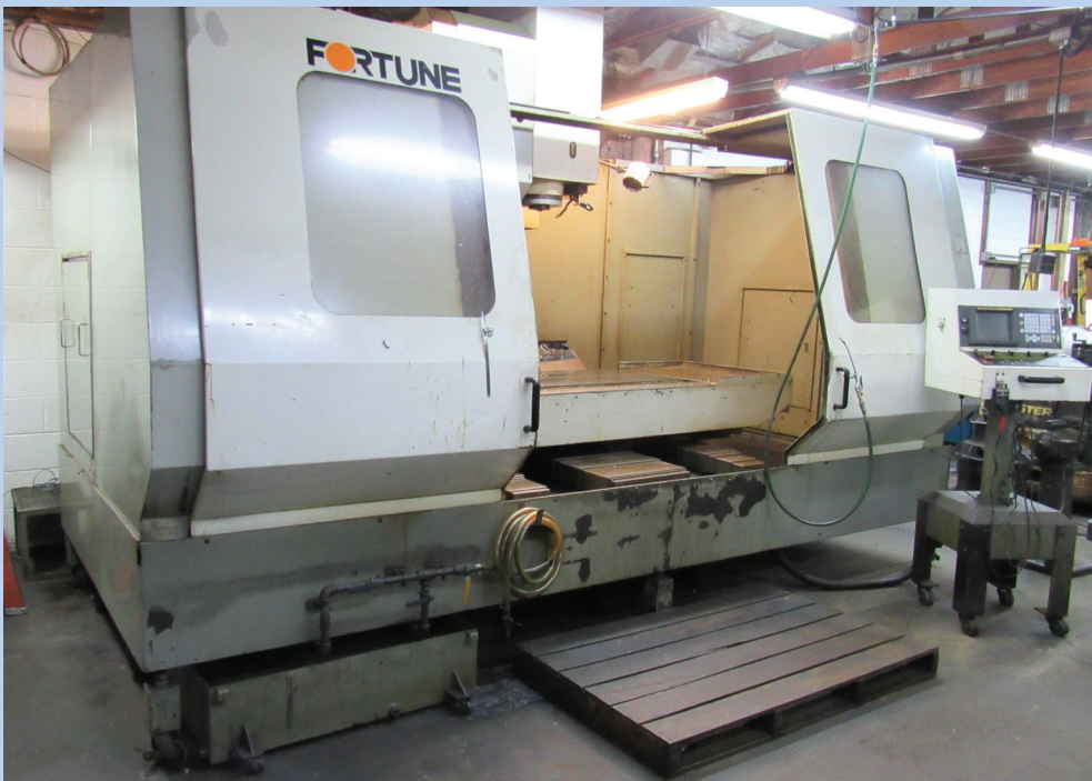
FORTUNE Model V-Center 140 Vertical Machining Center
